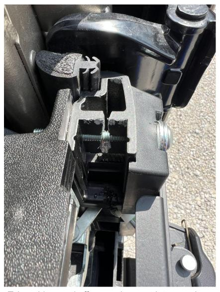
Take rubber seal off upper door, cut into rear door under rubber seal to get bolt out if square nut rounds off in plastic.
